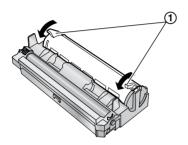
**10** Make sure that the triangles (①) match, to install the toner cartridge correctly.
